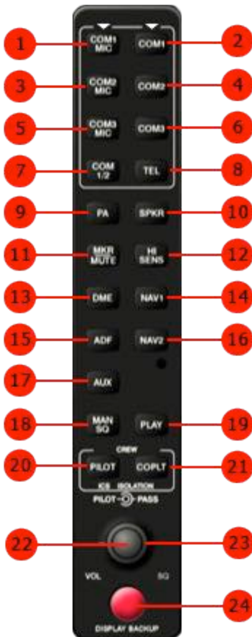
Audio Control Panel
